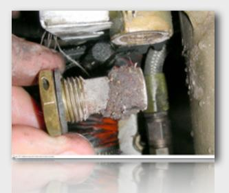
Besides rutile, the <u>rest was described</u> as cellulose material similar to wood or sawdust, thin metallic shavings, white flakes similar to paint, granular material like sand or dirt and fabric or glass fibers.
